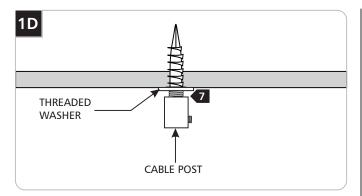
7 Screw the cable posts to the threaded washers.
