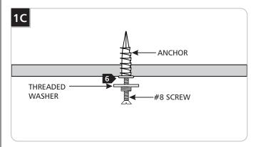
6 Attach the threaded washer to the anchors with the #8 screw.
