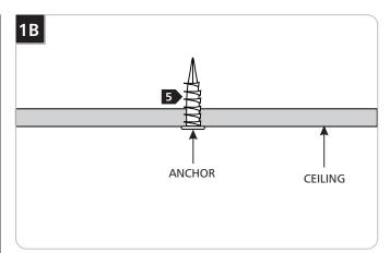
Screw the anchors in the rest of the way with a Phillips screwdriver.
