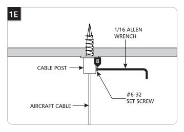
8 Feed the aircraft cables into the cable posts and tighten the #6-32 set screw with the 1/16 Allen wrench.
