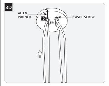
Push the excess power feed wires into the canopy and tighten the plastic screws with the provide Allen wrench.
