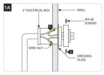
NOTE: 2" Electrical box should be installed prior to these steps. Refer to the instructions provided with the 2" electrical box.
