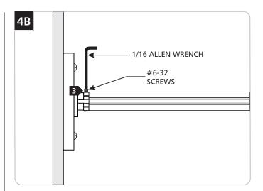
Tighten the #6-32 set screws on the conductive connectors with the provided 1/16 Allen wrench.
