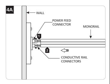
Insert the conductive rail joiners into the power feed connectors.
