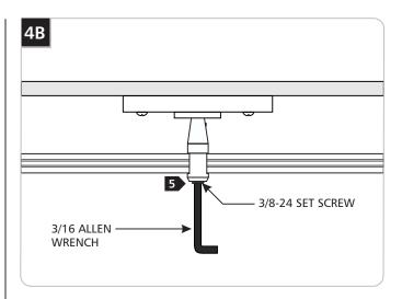
Tighten the 3/8-24 set screw on the bottom of the housing with the 3/16 Allen wrench.
