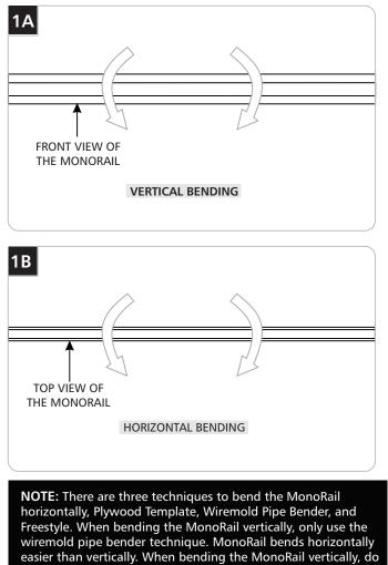
small bends at the time and avoid bending the MonoRail back which may cause the rail to separate from the insulator.
