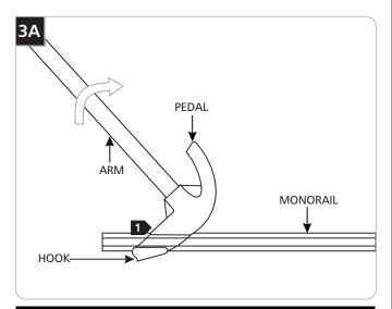
**NOTE:** The Wiremold pipe bender can be used to create smooth horizontal curve of 90° or less. Avoid stepping on the pedal of the pipe bender which will flatten and damage the MonoRail.
