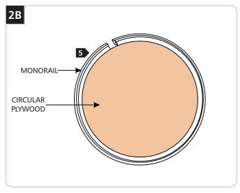
**5** Start bending the rest of the MonoRail against the circular plywood until the desired curve or circle is achieved.
