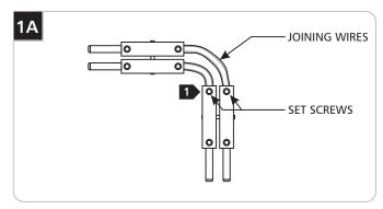
The joining wires on the flexible connectors are precut for a 90-degree bend. For any angle other than 90 degrees, follow these instructions to adjust the wires. Otherwise, skip ahead to section 2.
