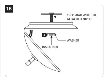
Remove the inside nut and washer to remove the crossbar with the attached nipple. DO NOT REMOVE the nipple from the crossbar.
