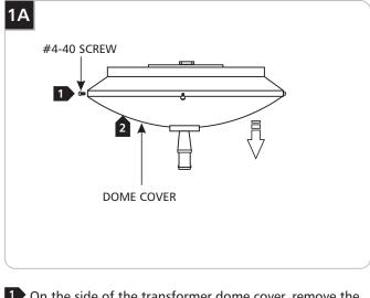
On the side of the transformer dome cover, remove the #4-40 screws with a Phillips head screwdriver.
