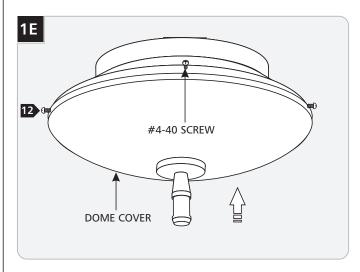
Replace the dome cover onto the transformer housing.Line up the dome cover holes with the transformer housing holes. Replace and tighten the #4-40 screws.
