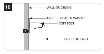
2 Use the large threaded washer when the Kable Lite cable is attached at an angle to the soft post.
