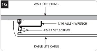
10 Insert one end of the Kable Lite cable into the soft post and tighten the three #6-32 set screws with the 1/16 Allen wrench to secure the wire. The other end of the cable should be attached to a turnbuckle.
