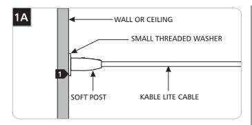
1 Use the small threaded washer when the Kable Lite cable is attached inline to the soft post.
