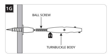
11 Screw the turnbuckle body to the ball screw.
