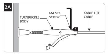
**NOTE:** When power feed wires are going to be connected to the turnbuckle bodies (Fig 3A on page 3) and insulated Kable Lite cables are used in the system, strip the end portion of the Kable Lite cables (that are going to be attached to the turnbuckle bodies) so that the power is conducted through the turnbuckle bodies to the Kable Lite cables. This does not apply for isolated slimline turnbuckles.
