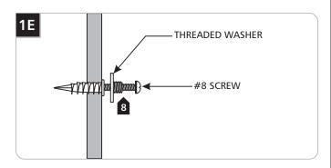
8 Attach the threaded washer to the anchor with the #8 screw.
