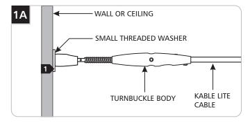
1 Use the small threaded washer when the Kable Lite cable is attached inline to the soft turnbuckle.
