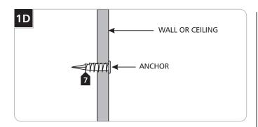
Screw the anchors in the rest of the way with a Phillips screwdriver.
