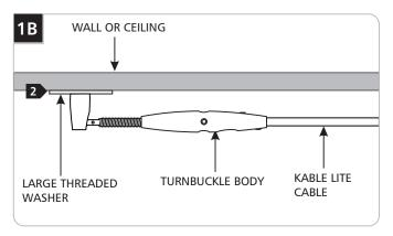
2 Use the large threaded washer when the Kable Lite cable is attached at an angle to the soft turnbuckle.
