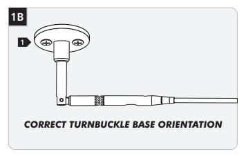
1 When mounting the universal turnbuckle onto the ceiling or at an angle, make sure that the turnbuckle base is in correct orientation (screw holes being inline with the Kable Lite cable).
