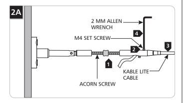
**NOTE:** When power feed wires are going to be connected to the turnbuckle bodies (Fig 3A on page 3) and insulated Kable Lite cables are used in the system, strip the end portion of the Kable Lite cables (that are going to be attached to the turnbuckle bodies) so that the power is conducted through the turnbuckle bodies to the Kable Lite cables.
