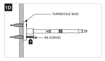
Mount the turnbuckles to the anchors through the turnbuckle base holes with the #8 screws.
