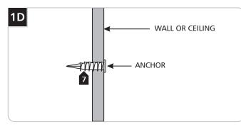
Screw the anchors in the rest of the way with a Phillips screwdriver.
