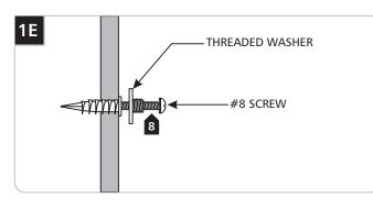
8 Attach the threaded washer to the anchor with the #8 screw.
