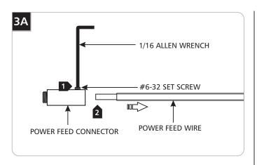
Loosen the #6-32 set screw on the power feed connectors with the 1/16 Allen wrench.
