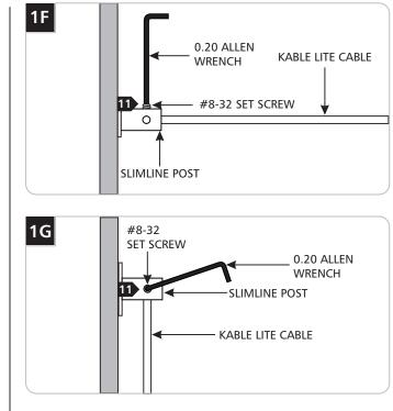
Insert one end of the Kable Lite cable into the slimline post and tighten the #8-32 set screws with the 0.20 Allen wrench to secure the wire. The other end of the cable should be attached to a turnbuckle.
