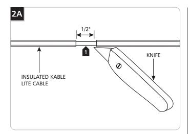
When using insulated Kable Lite cables, remove 1/2" of the insulation from each cable (where the power feed connector is going to be mounted) with a sharp knife. Make sure not to cut or nick the cable.
