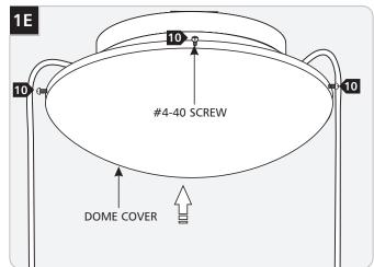
Replace the dome cove onto the transformer housing. Line the dome cover holes up with the transformer housing holes. Replace and tighten the #4-40 screws.
