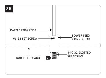
2 Unscrew the #10-32 slotted head set screw from the tip of the power feed connectors with a screwdriver. Place the power feed connectors one onto each Kable Lite cable and tighten the #10-32 slotted set screw on the tip with the screwdriver.
