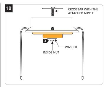
Remove the inside nut and washer to remove the crossbar with the attached nipple. **DO NOT REMOVE** the nipple from the crossbar.
