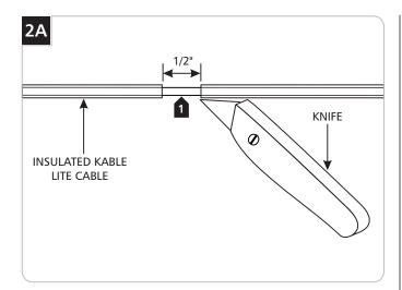
When using insulated Kable Lite cables, remove 1/2" of the insulation from each cable (where the power feed connector is going to be mounted) with a sharp knife. Make sure not to cut or nick the cable.
