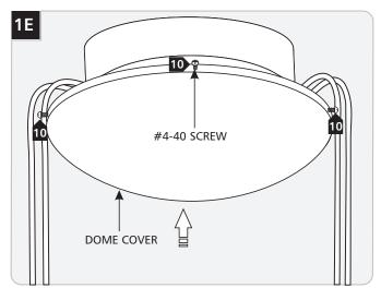
Replace the dome cove onto the transformer housing. Line up the dome cover holes with the transformer housing holes. Replace and tighten the #4-40 screws.
