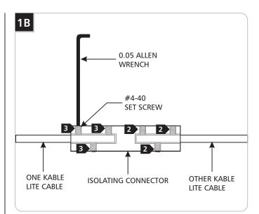
Feed end of one Kable Lite cable half way into the side hole of the isolating connector and tighten the three #4-40 set screws with the 0.05 Allen wrench.
