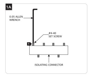
Loosen (Do Not Remove) the six #4-40 set screws with the provided 0.05 Allen wrench to clear the side holes.
