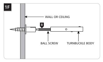
8 Screw the turnbuckle body to the ball screw.
