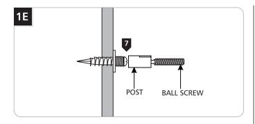
**7** Screw the post with the ball screw onto the threaded washer.
