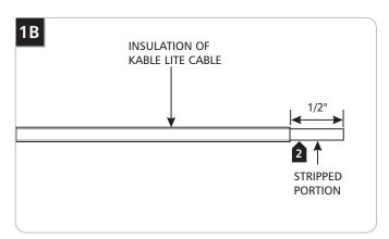
When using the insulated Kable Lite cables, strip 1/2" of insulation from end of the cables feeding into the conductive connectors.
