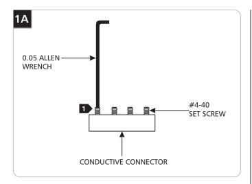
Loosen (Do Not Remove) the four #4-40 set screws with the provided 0.05 Allen wrench.
