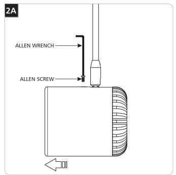
1 If installing or replacing lens accessory or replacing the optic, remove the cover by unscrewing the Allen screw from the top of the fixture using the provided Allen wrench.
