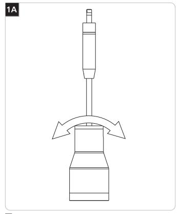
1 Tilt the fixture head to the desired position.
