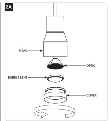
**NOTE:** While installing or replacing lens and/or optics, it is recommended to do so with the fixture head facing downward to hold items in place within the cover during installation.
